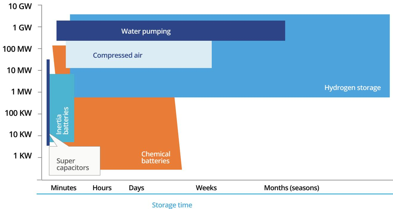
Figure 1-12 shows a technological map to choose between energy storage options according to the volume of energy, storage time, and technical capabilities.
